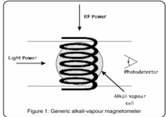
Figure 1: Generic alkali-vapour magnetometer
