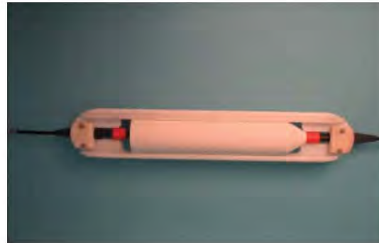
New OhmMapper Connector Protectors Ideal for towing the OhmMapper over rough surface conditions.
