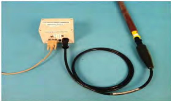
Data logging box connected to serial cable Can also be used with a Bluetooth Adaptor to connect to an Android phone or tablet.
