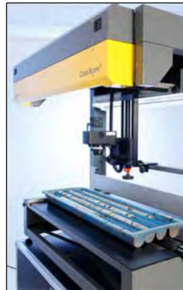
Scanning of Slabbed Core and Core Boxes
