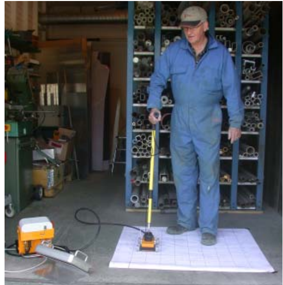
Figure 3. Data acquisition using grid carpet. The entire data collection process may be steered completely by remote controls located on the extension handle.
