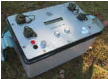
Extension Switch Pro box able to drive 24 - 48 - 72 or 96 electrodes
